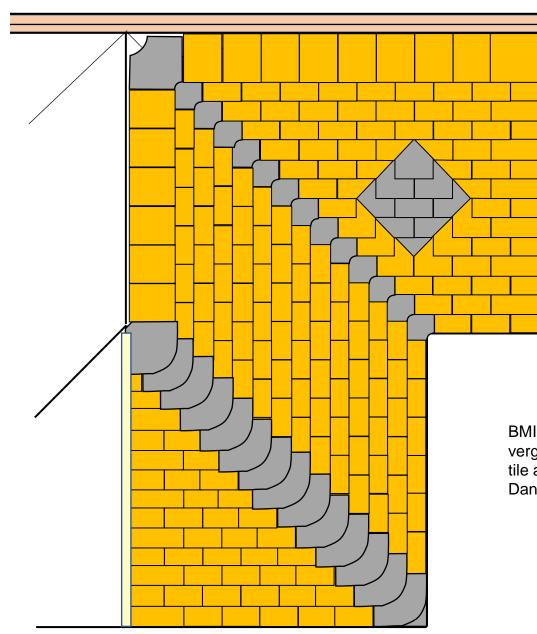
BMI concrete plain tiles hip and valley to a wet verge detail incorporating purpose made valley tile and bonnet hip tiles and Hambleside Danelaw GRP soakers to the abutment
