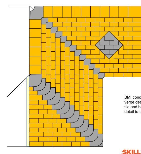
BMI concrete plain tiles hip and valley to a wet verge detail incorporating purpose made valley tile and bonnet hip tiles. Form a small diamond detail to the valley to verge section
